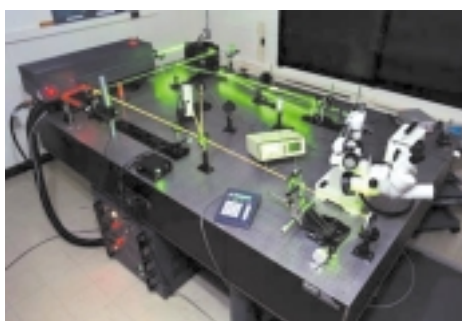
The optical damage threshold test station at NASA Langley Research Center has three lasers: ND:Yag laser, a Ti:Sapphire laser, and an He Ne laser.
