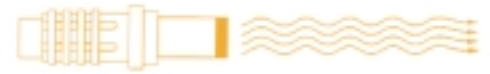
COHERENT or MONOCHROMATIC — LASER Same wavelength (monochromatic) Light waves in phase (coherent)
