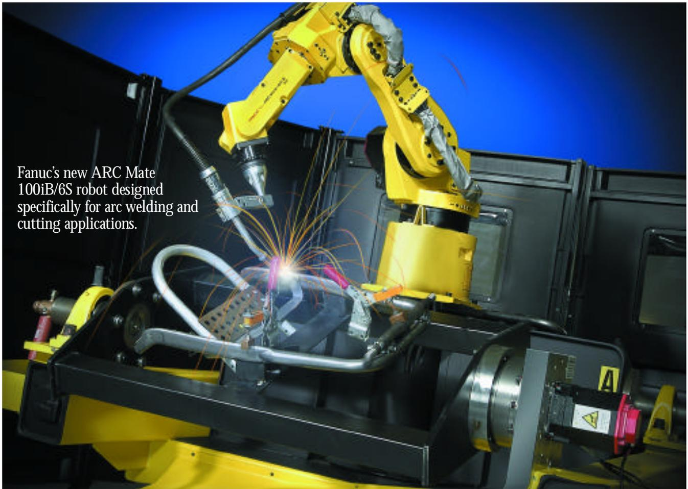
Fanuc's new ARC Mate 100iB/6S robot designed specifically for arc welding and cutting applications.
