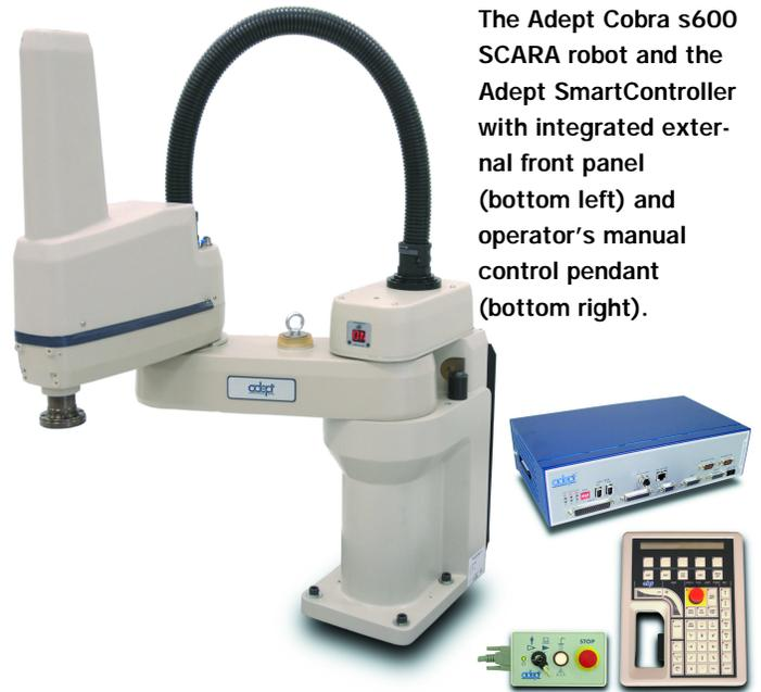
The Adept Cobra s600 SCARA robot and the Adept SmartController with integrated external front panel (bottom left) and operator's manual control pendant (bottom right).
