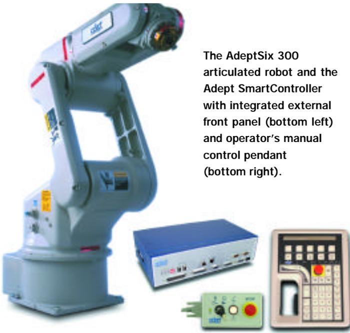
The AdeptSix 300 articulated robot and the Adept SmartController with integrated external front panel (bottom left) and operator's manual control pendant (bottom right).
